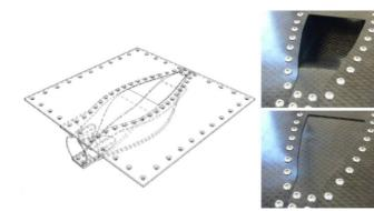
Morphing structures are structures that change shape or state in order to change their operating characteristics or as a response to changes in environmental conditions. Bistable structures are good candidates to be used as morphing structures because they have ability to remain in equilibrium in two predefined shapes. Actuation is required to transit, 'snap-through,' between these stable states.
